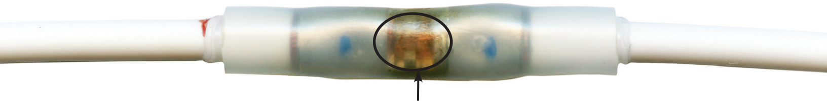
Window is visible with some red dye remaining in window
